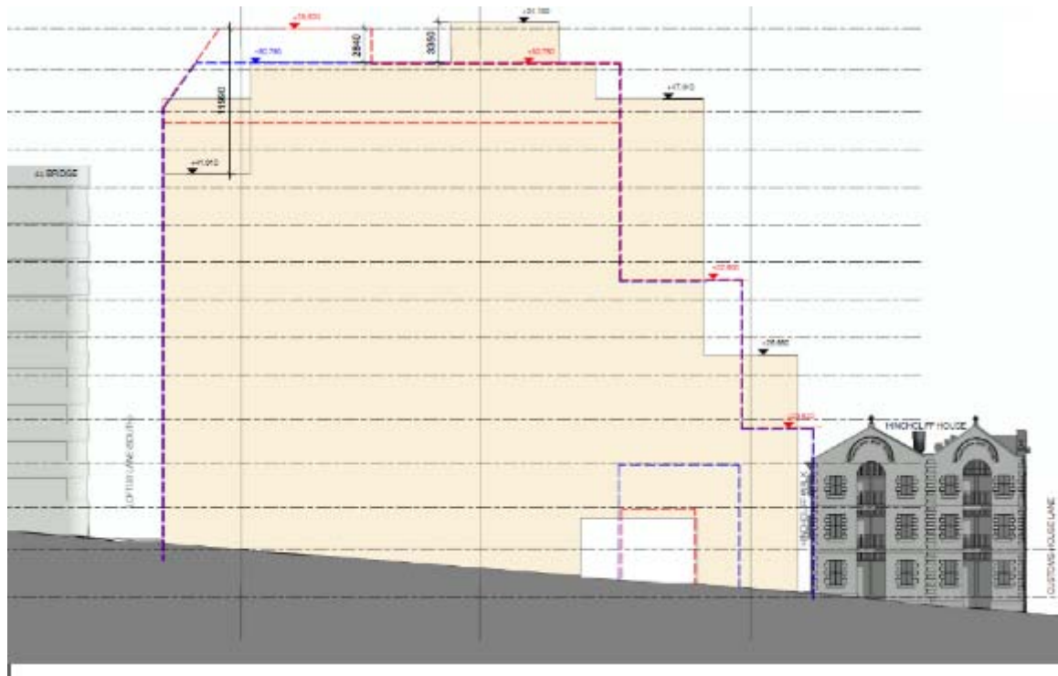
Figure 21: Building C – proposed built form shaded and dotted lines are approved building envelopes (blue line – Stage 1 approval, red line – DCP building envelope).
